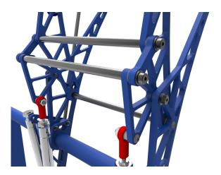
The steep angle is used while close to the goals and truss shots. The shallow angle is used other shots from farther away or while moving.
