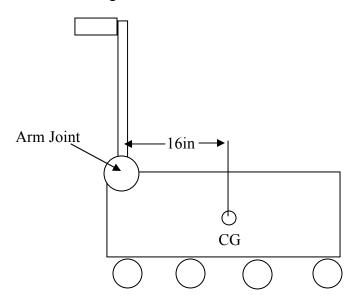
For the robot weight, 150 lbs is assumed, located at the CG.
