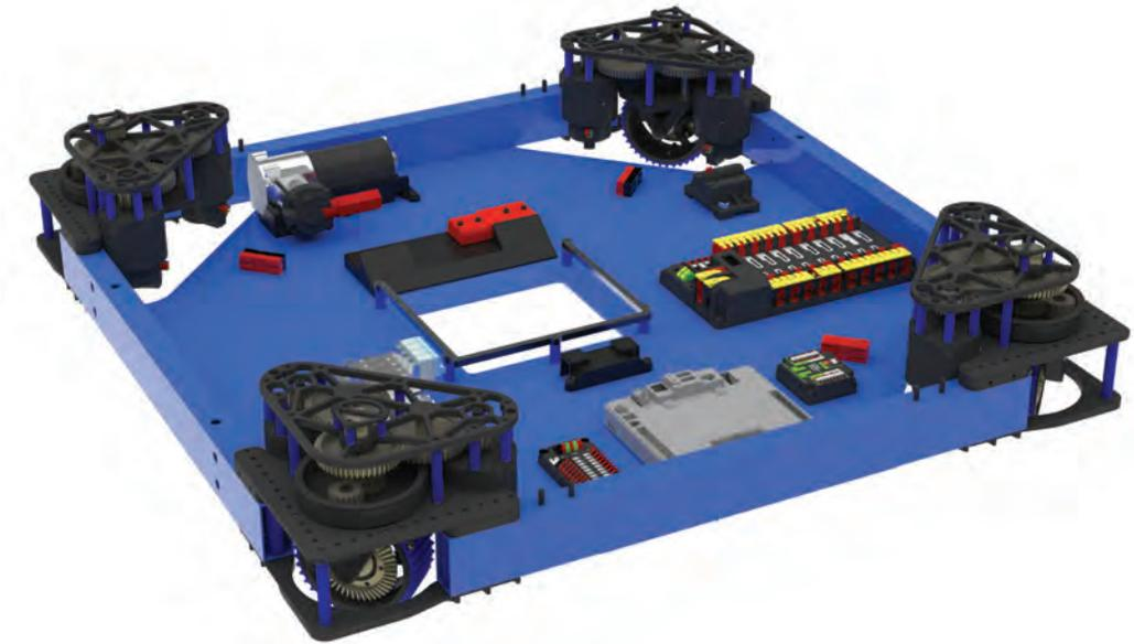
The drivebase allows the robot to maneuver around the field quickly and precisely. Unlike the past 20 years of West Coast Drives, this year features Team 254's first-ever swerve drive. The swerve was chosen for its increased maneuverability and ability to avoid defense.
