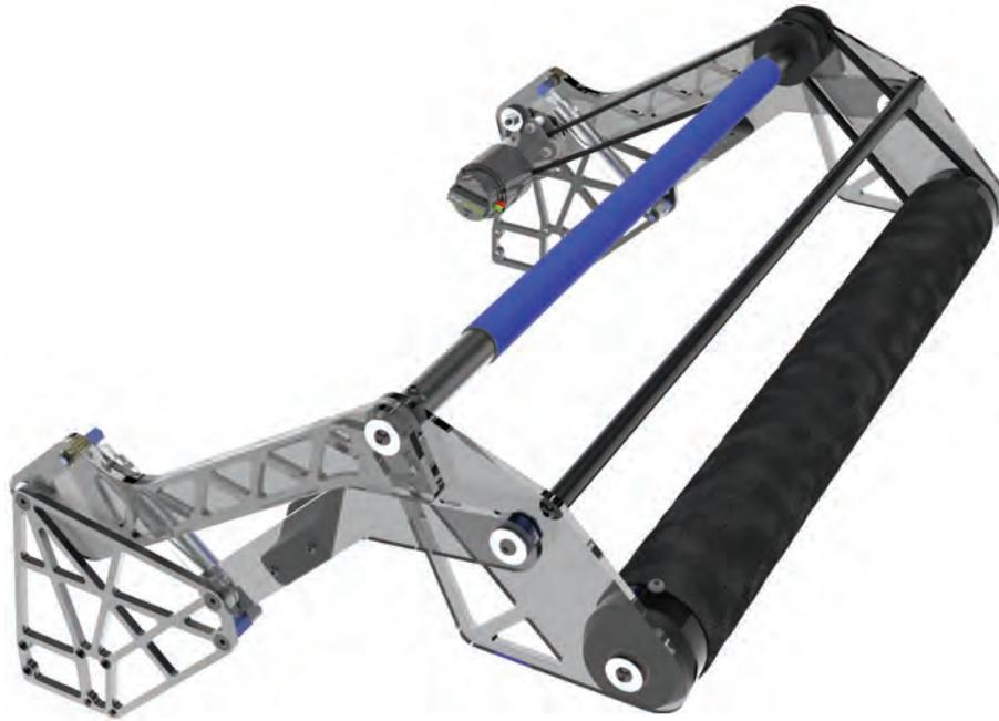
The two intakes pull balls from the ground over the bumper into the Serializer. Robot-width horizontal rollers on a pneumatically actuated four-bar create a robust touch-it-own-it mechanism.
