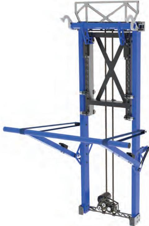
The Elevator and Reaction Arm are the first components of the inventive and fast climber. The Elevator grabs the second bar and pulls down until the Reaction Arm hits the underside of the truss and tilts the robot to level, allowing the Stinger that is just within the extension limits to reach the traversal bar. The exceptional forces (500+ lbs) generated during this maneuver made for a challenging design!
