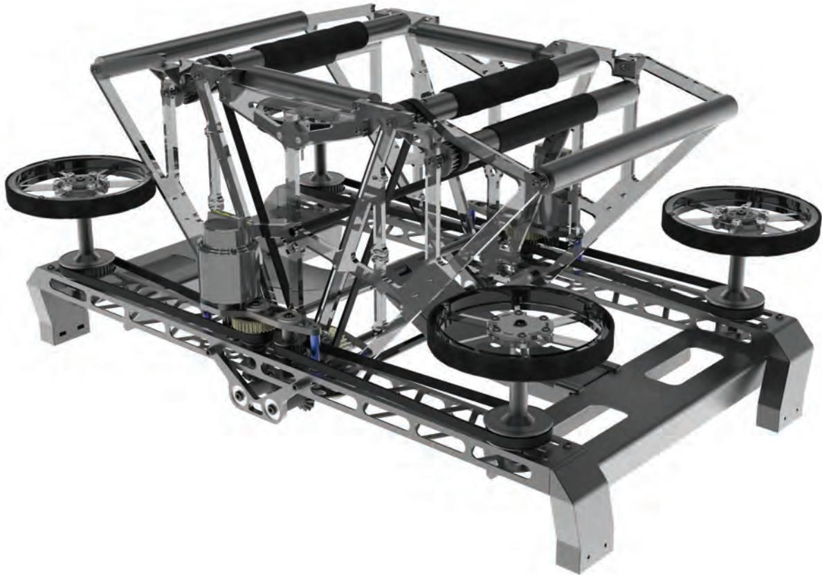
The Serializer funnels balls from the dual 30" wide intakes into a single stream to feed into the Shooter. Color sensing enables the Serializer to store our balls while ejecting opponents'.
