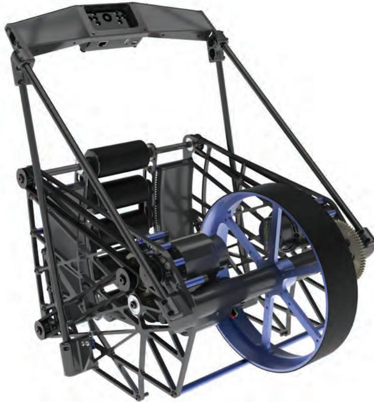
The high accuracy and large shooting range requirements drove the need for a flywheel shooter with a lot of grip, wrap (acceleration time), and an adjustable hood.
