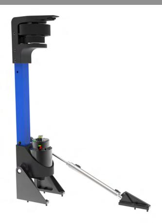
The "Wheel of Fortune" (WOF) Mechanism is a pneumatically deployed arm with a wheel and color sensor at the top to manipulate the Control Panel.
