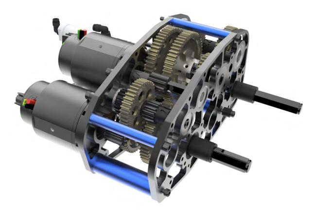
The drive gearbox provides the reduction from the drive motors to the wheels to power the drivetrain. This year's drive gearbox has two speeds and contains a Powered Take-Off for the climber.
