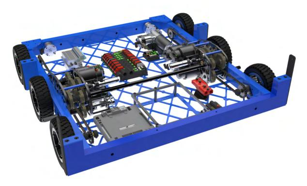
The drivetrain allows the robot to maneuver around the field quickly and precisely. This year's design is a "West Coast Drive" which features pneumatic wheels and a square drivetrain. The simplicity, reliability, and power of the WCD has served us for many years. For this reason, we could expend more effort and resources working on other subsystems.
