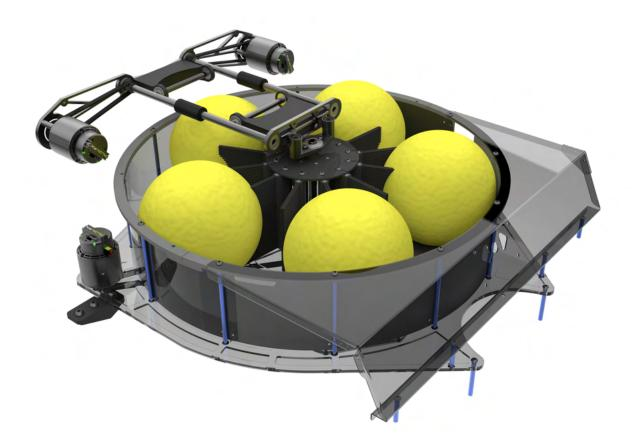
The serializer receives up to 3 balls from the intake and indexes up to five balls so that they can be shot rapidly without jamming. The feeder pulls balls out of the serializer circle and into the shooter.
