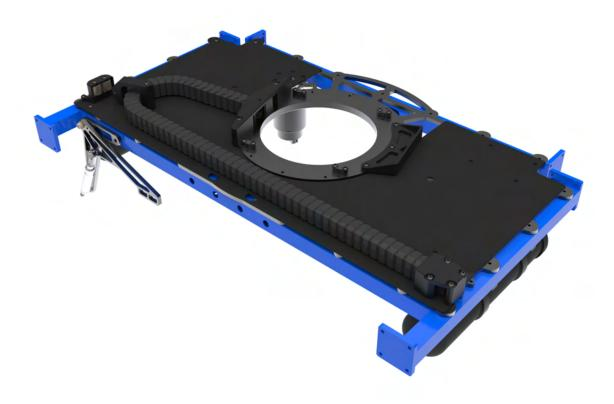
The turret sits above the serializer and rotates the shooter so that the robot can quickly score balls from nearly any orientation. It is powered by a Falcon 500 and uses a horizontal bidirectional IGUS chain for wire management.
