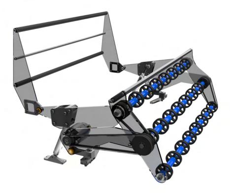
Our team's philosophy for intake design is "Touch it, own it." This year's intake consists of 3 robot-width horizontal rollers on a pneumatically actuated four-bar to lift up to 3 balls over the Bumper and into our Serializer.
