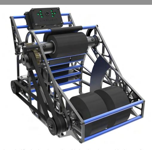
The shooter utilizes dual-flywheels with an adjustable hood angle to enable shooting from a majority of the field locations. A Limelight camera on top vision tracks retro-reflective tape on the goal to aim the turret, control the hood angle, and adjust the flywheel speed.
